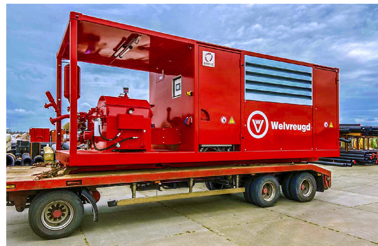
P2500E6650 2500 l/min a 100 bar | 6000 x 2440 x 2600 mm (LxLxA) | 14000 kg
