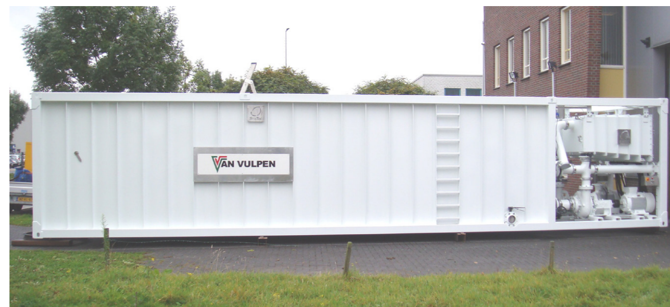
M4000E 4000 l/min | 12000 x 2450 x 2600 mm (LxLxA) | 9000 kg
