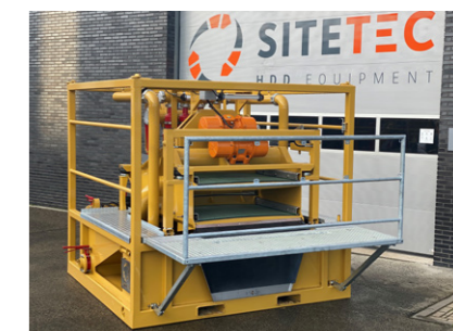
R500E compact 500 l/min | 2500 x 2500 x 2300 mm (LxLxA) | 3830 kg
