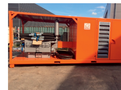
P1500D 1500 l/min a 70 bar | 6220 x 2350 x 2560 mm (LxLxA) | 8500 kg
