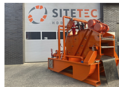
R250E compact 250 l/min | 2250 x 1600 x 2000 mm (LxLxA) | 2500 kg
