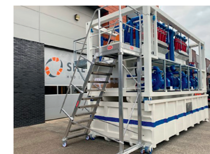
R2000E compact 2000 l/min | 6000 x 2450 x 2580 mm (LxLxA) | 9800 kg
