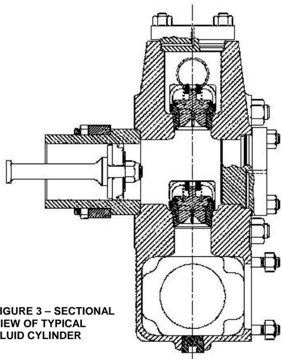
**FIGURE 3 – SECTIONAL VIEW OF TYPICAL FLUID CYLINDER**
