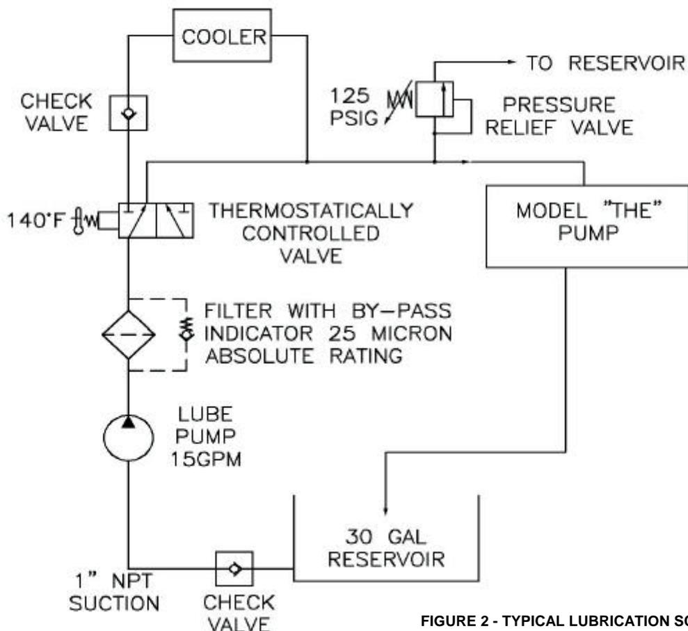
FIGURE 2 - TYPICAL LUBRICATION SCHEMATIC
