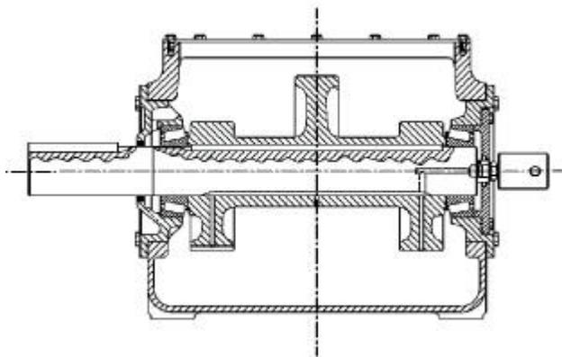
FIGURE 4 – SECTIONAL VIEW SHOWING ECCENTRIC
