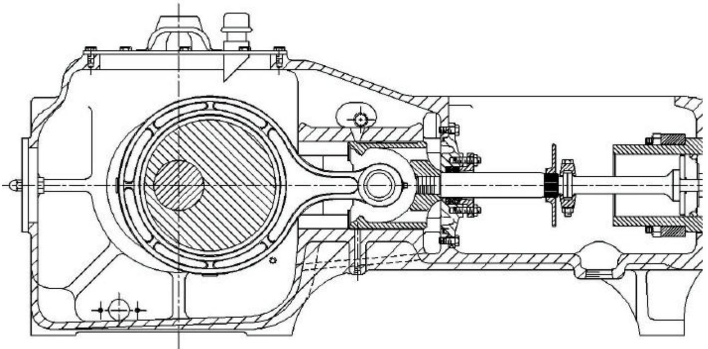
FIGURE 1 – SECTIONAL VIEW OF MODEL 'THE' TRIPLEX PISTON PUMP
