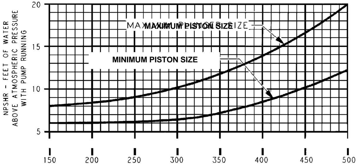
Pump Bulletins list the maximum and minimum piston sizes.
