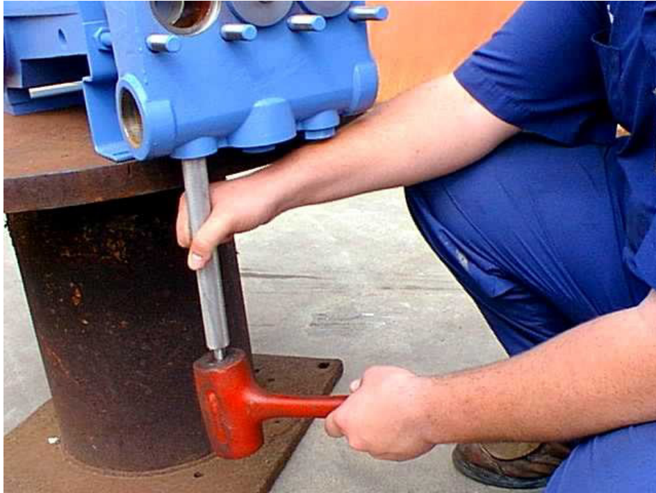
Figure 7: Removing the valve from the seat
