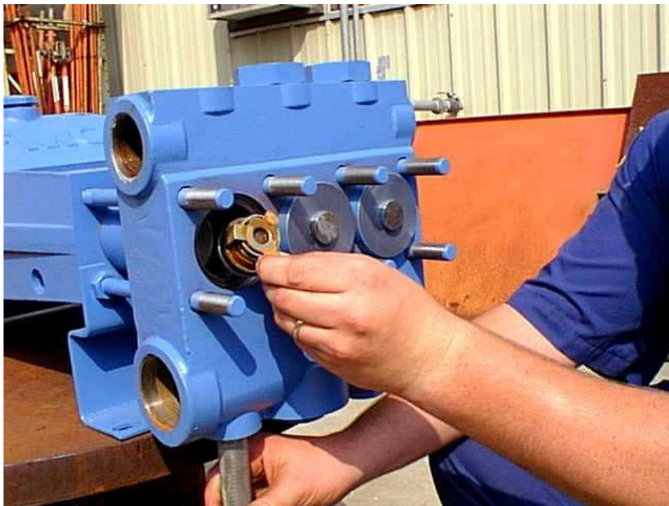
Figure 8: Removing the valve from the fluid cylinder
